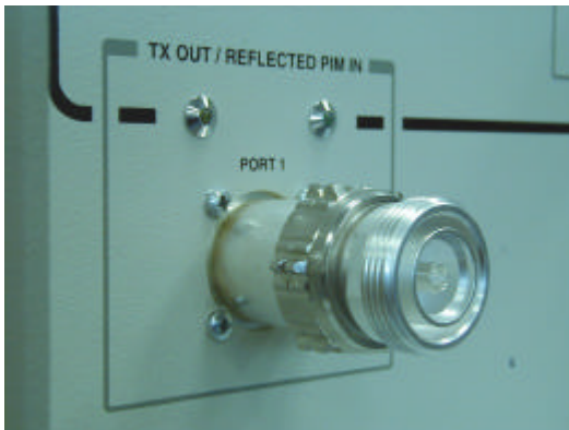
Figure 1. Front Panel 7-16 Connector with Connector Saver
